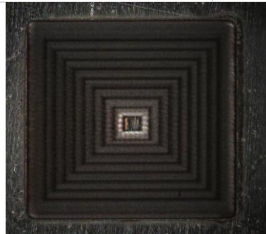
Optical microscope image (left), 3D profiler images (middle) and 2D profiler profiles (right) of 3D cavity engraved in stainless steel by laser-polygon duet system.
