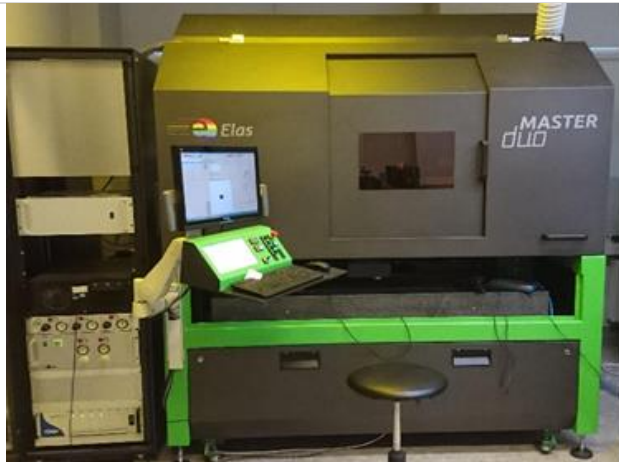
DuoMaster laser processing system of ELAS in FTMC lab.
