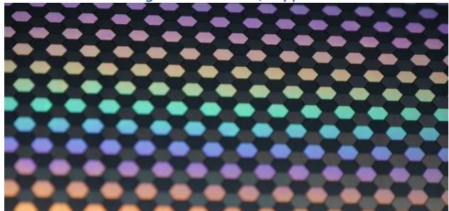
Micrometre size structure with additional optical active nanometre size structures, chromium sleeve.
