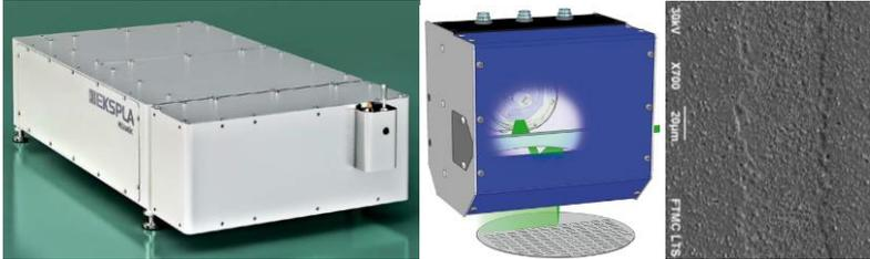
Picosecond laser Atlantic (Ekspla) and polygon scanner LSE 170 (Next Scan Technologies) provide opportunity to reach the removal of the full CIGS structure to expose the molybdenum back-contact at the scribing speed of 50 m/s.
