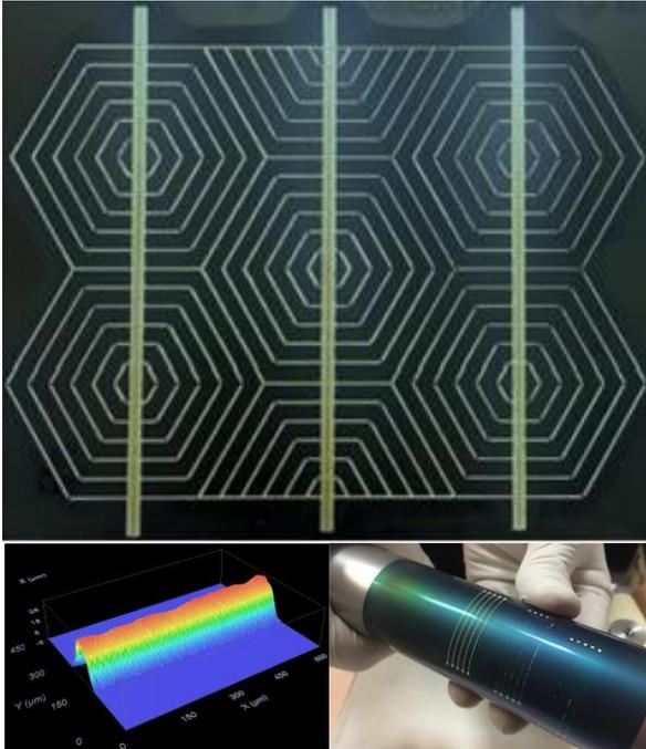
This allows the printing of different grids just changing the program for the scanner giving great process flexibility.
