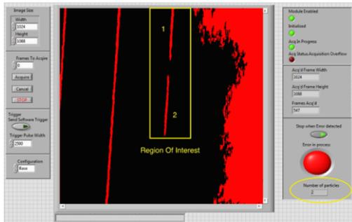
With a high speed camera (max 500 fps), recognition of the defects was achieved at the maximum speed of 1100 mm/s. This was demonstrated for CIGS P3 type 1, Cr/Glass P1 and Mo/PI P1 processes.
