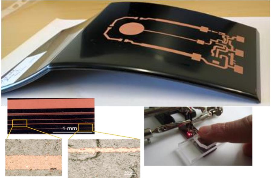
*Selectively plated copper on Polypropilene surface and functional capacitive sensor demonstrator.*
