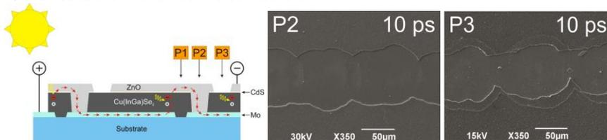
Schematic view of the CIGS module series interconnect formed with three step laser scribing. SEM images of the P2 and P3 lift-off scribes in CZTSe samples.
