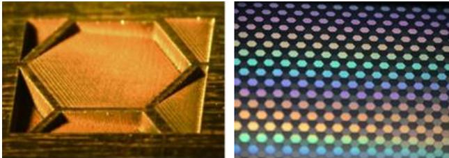
Laser processing with ultra-short laser pulses gives the possibility for texturing of surfaces with sub-micrometre size structures. Due to the small, size these structures are optical active and give the product designers an unexplored option in terms of appearance and functionality.
