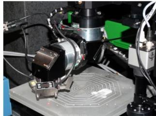
*Add-ins to DuoMASTER laser system (ELAS): roll-to-roll setup and robotic hand for 3D processing.*
