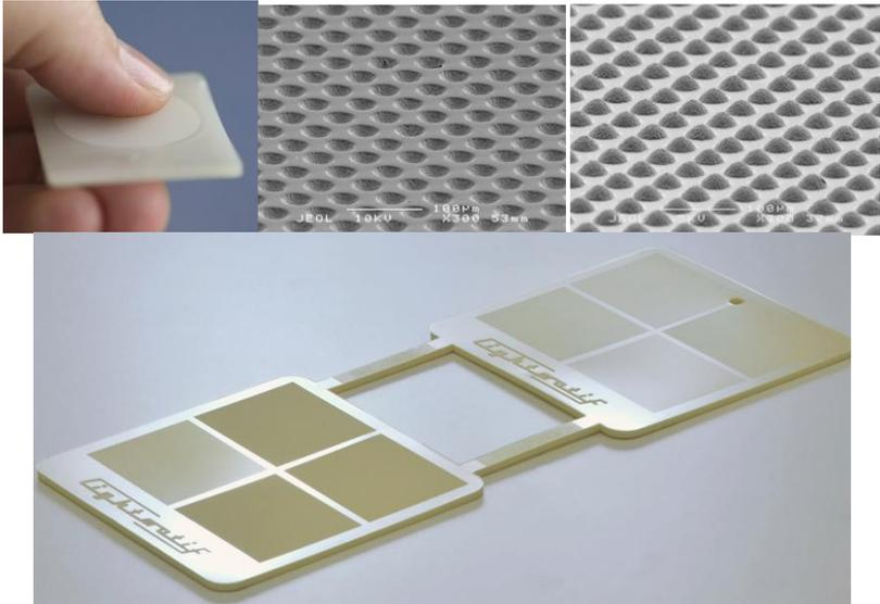
*SEM images of dimples produced by laser trepanning and their replicas made by injection moulding. Injection moulded demonstrator with different soft-touch / anti-glare micro-pillar textures.*
